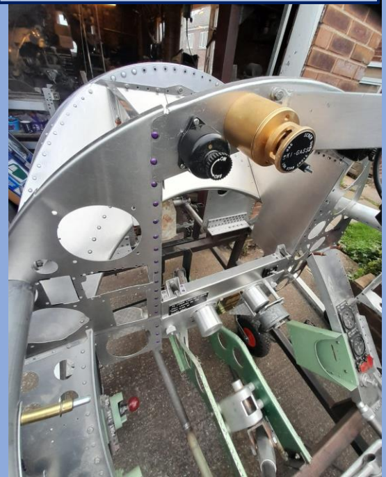
Cockpit stripped out, windscreen and top coamings off, half way through the big rivet.
