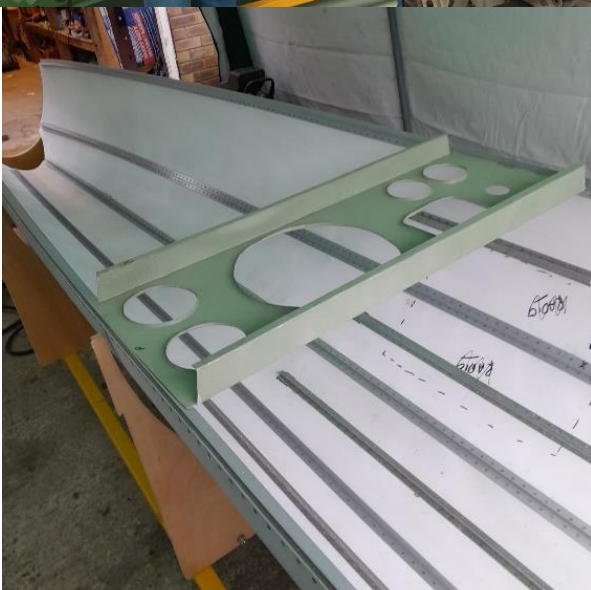
The IFF instrument tray in place to check dimensions.
