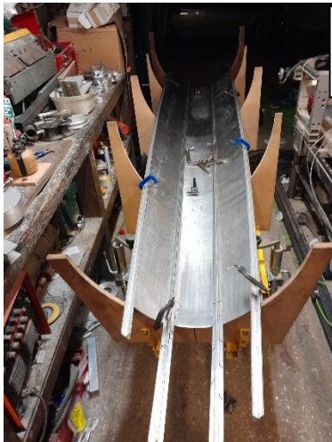
Trimmed panels and stringers coming together in the cradle.
