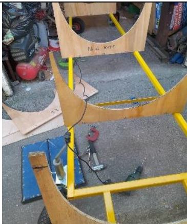
Assembling the lower fuselage cradle.
