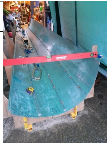
Trimmed panels and stringers coming together in the cradle.
