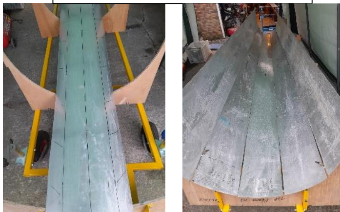
Laying out the lower skins for trimming.
