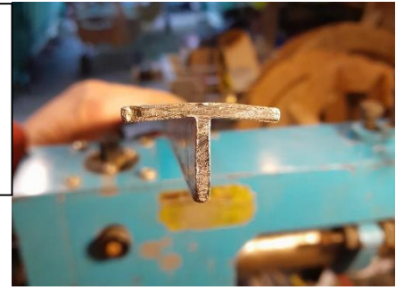
T-stringers after rolling for the correct radius profile.
