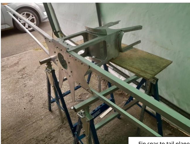
Fin spar to tail plane spar connector plate – along with the very long spar booms.
