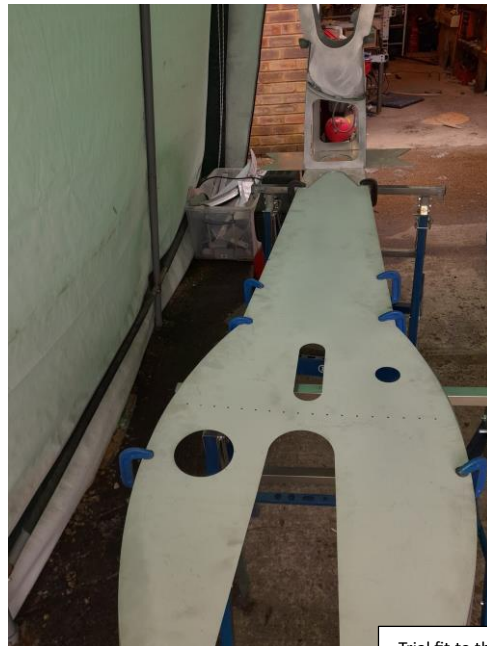
Trial fit to the tail fin – at the workshop.
