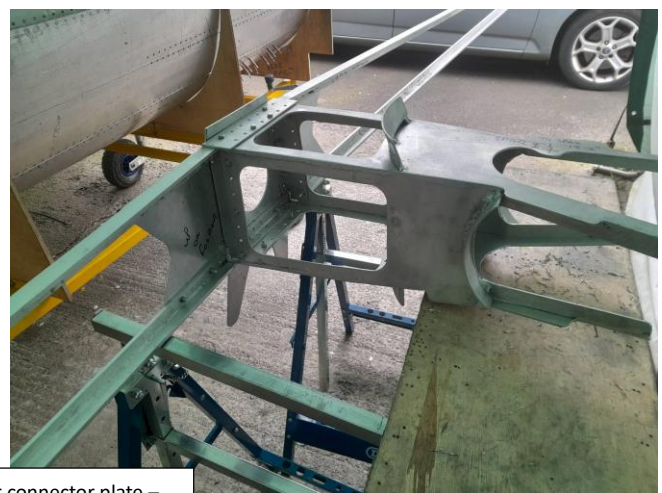
Fin spar to tail plane spar connector plate – along with the very long spar booms.
