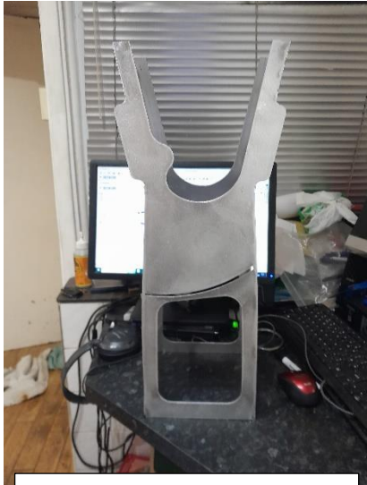
Fin and tail plane connector – manufactured in separate parts and welded together.
