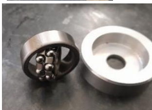
Special self-aligning bearings for the rudder.
