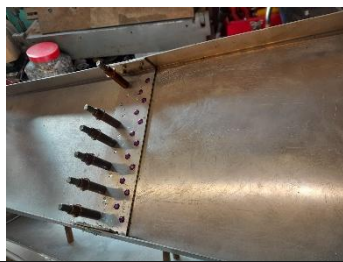
Rudder spar cut out – strengthening plates added – trial fit with upper and lower pivot arms. See 2025 Spring newsletter!
