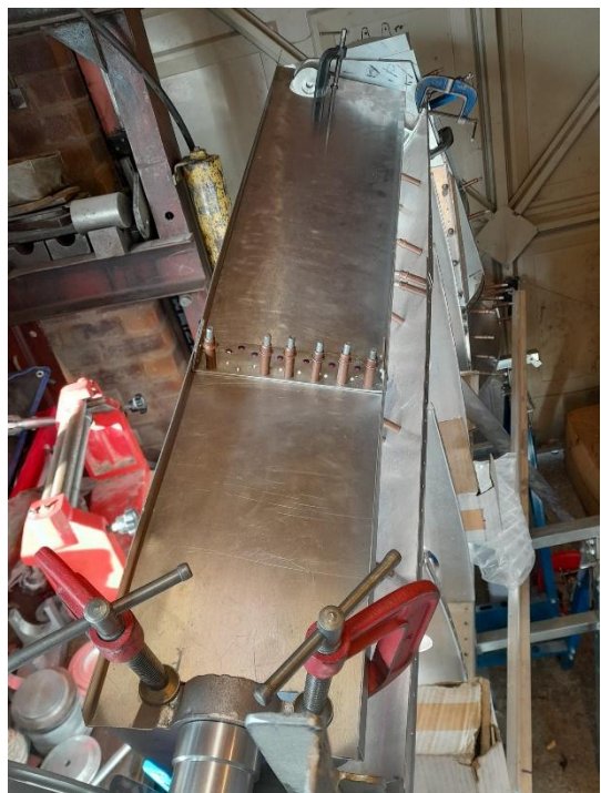
Rudder spar cut out – strengthening plates added – trial fit with upper and lower pivot arms. See 2025 Spring newsletter!
