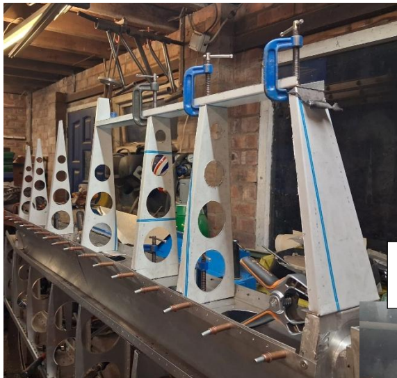
The elevator rear spars, that accommodate the trim tabs make an appearance...
