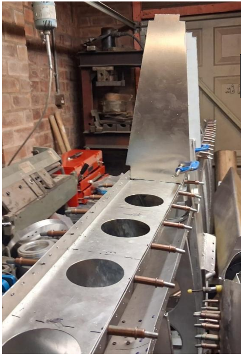
Green-fitting the ribs and auxiliary spars. It's building up to be an impressive structure.
