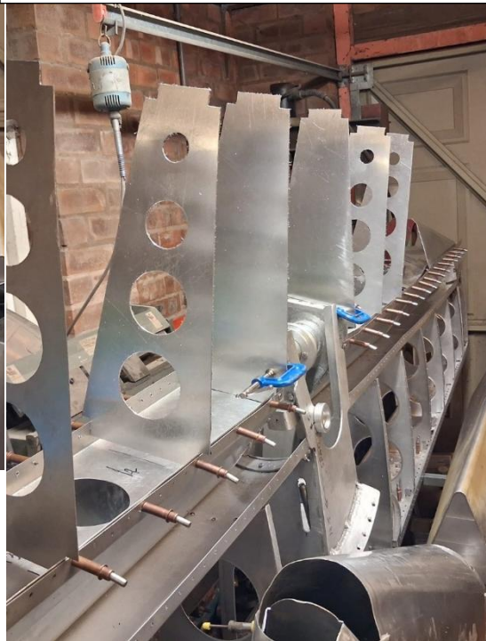
Green-fitting the ribs and auxiliary spars. It's building up to be an impressive structure.
