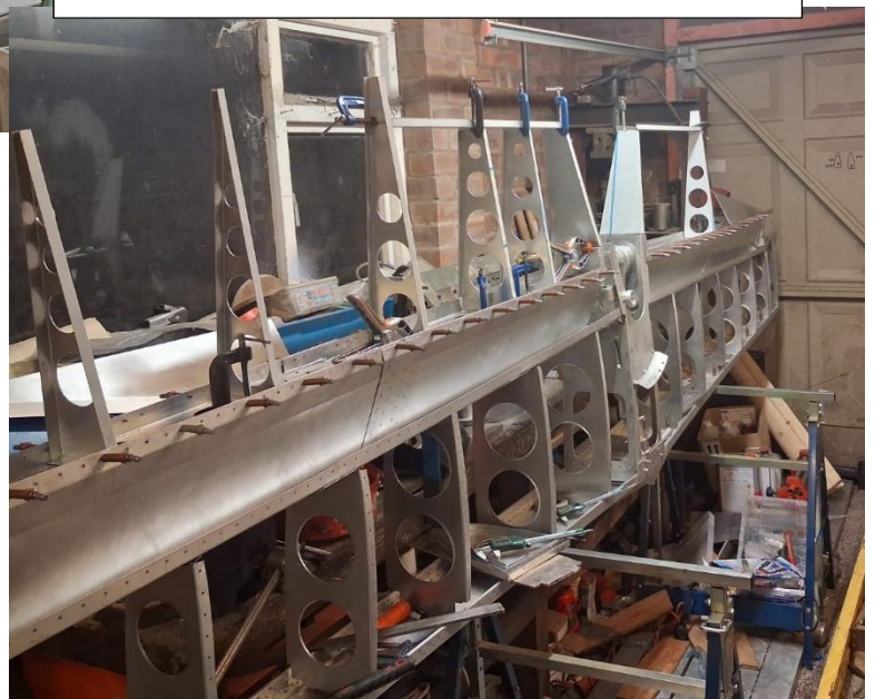
The elevator rear spars, that accommodate the trim tabs make an appearance...
