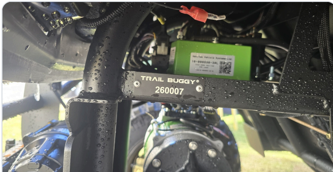
Serial plate · Front of chassis, left / driver side — Trail Buggy® plate shows your serial (example shown: 260007).
