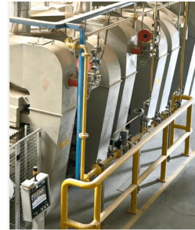
Primus gas-fired furnace, the process being replaced
