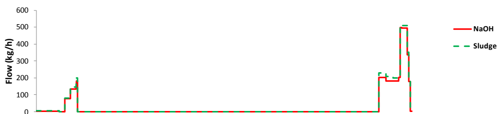
Figure C.3: Result of the calculation – NaOH consumption and sludge production.
