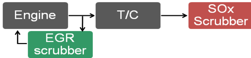
Figure 25: Simplified layout of combined EGR and EGC scrubber
