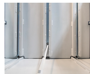
Compaction against counterplate by horizontal moving press ram
