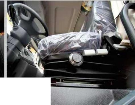
Four point air suspended auto-adjusting seat design according to man-machine curve, providing its occupants with superior quality and comfort. The seat is effective in reducing driver fatigue which ensures the driver have a safe and comfortable journey.
