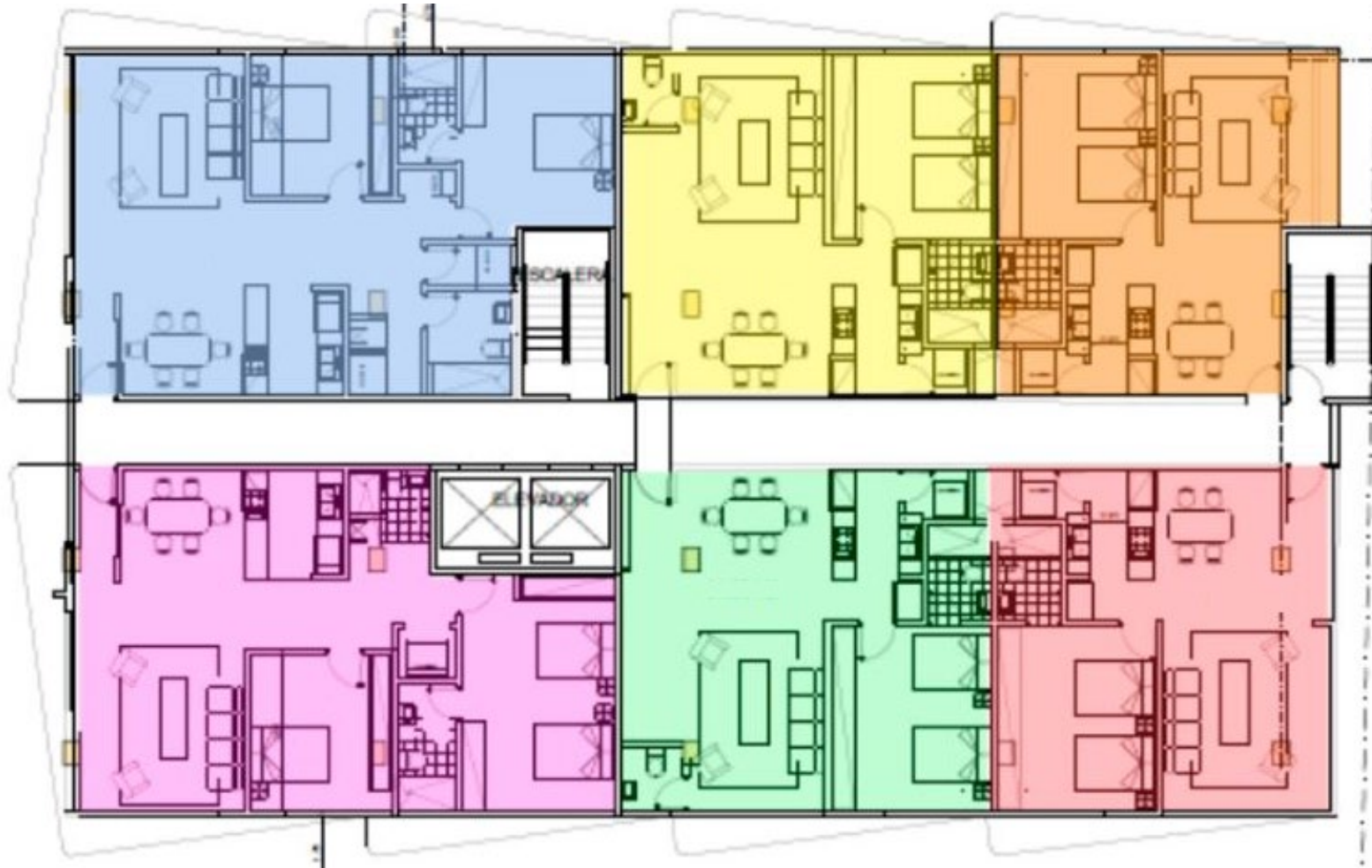
ARCHITECTURAL FLOOR PLAN 2 TO 15 LEVEL (TYPICAL)
