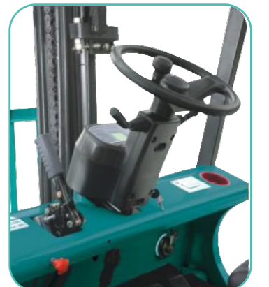
TILT ADJUSTABLE STEERING WHEEL CAN BE TILTED TO SUIT THE BEST WORKING POSITION FOR EACH OPERATOR.
