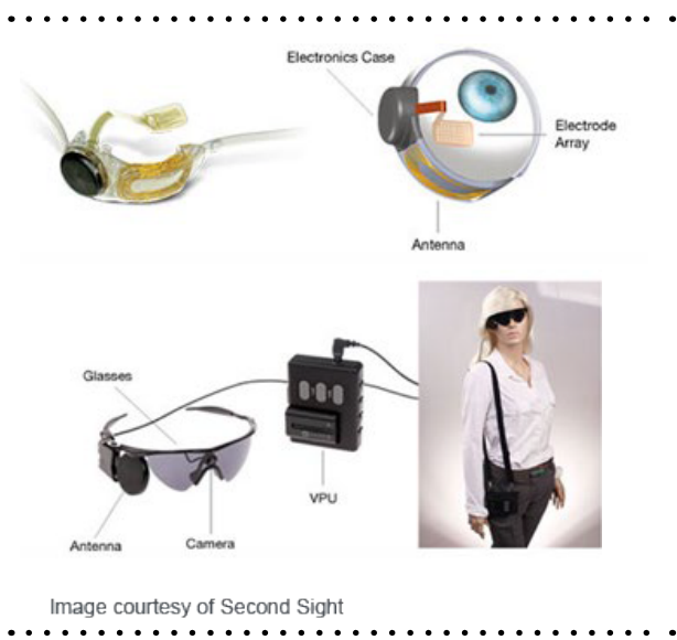
Figure 47 | The Argus II system (Source: https://chicago.medicine.uic.edu/argus-ii-retinal-prosthesis-system-on-trial-at-the-ieei/ )
