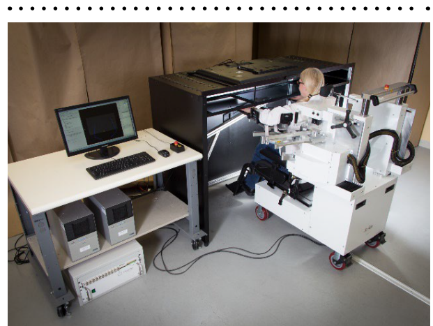
..... Figure 53 | The Kinarm rehabilitation training platform (Source: https://kinarm.com/kinarm-products/kinarm-exoskeleton-lab/ )
