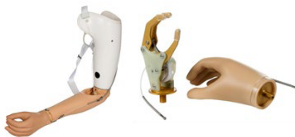
Figure 44 | Body-powered arm and hand (Source: https://www.ottobockus.com/prosthetics/upper-limb-prosthetics/solution-overview/body-powered-prosthetic-solutions/ )
