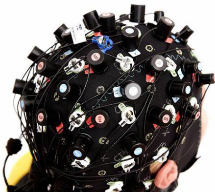
Figure 36 | The NIRSports device developed by NIRX, which can be scaled to high-density arrangement with 48 Sources and 48 detector arrangement with 3 connected fNIRS NIRSport2 devices (Source: NIRSports)
