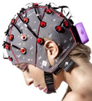
Figure 30 | The g.Nautilus EEG amplifier developed by g.tec (Source: g.tec)
