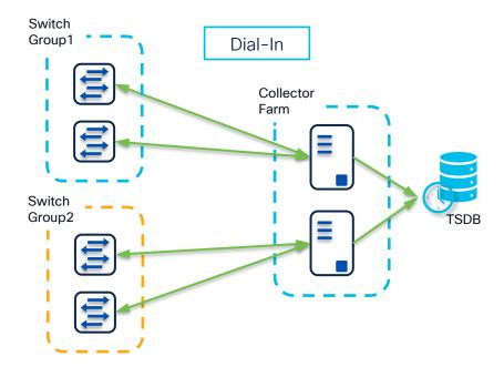
To distribute the workload, the collectors need to dial-in to different switch groups, need to keep the sensor configuration synchronized across the cluster
