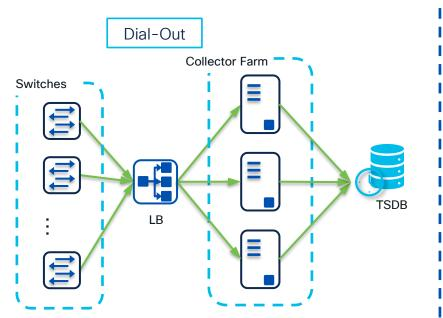
Collectors can be set up behind load balancer, all switches stream to the same VIP of collector
