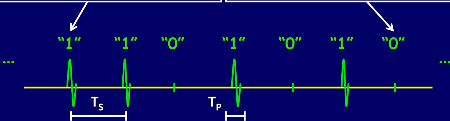
**Pulses are spread in time to simplify the transceiver architecture...**
