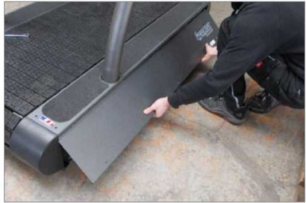
Fig. 23 4Front assembly, side panel
