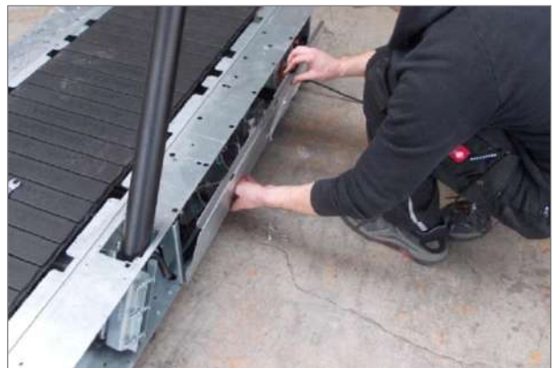
Fig. 47 Mercury/Path Assembly, electronic cover plate
