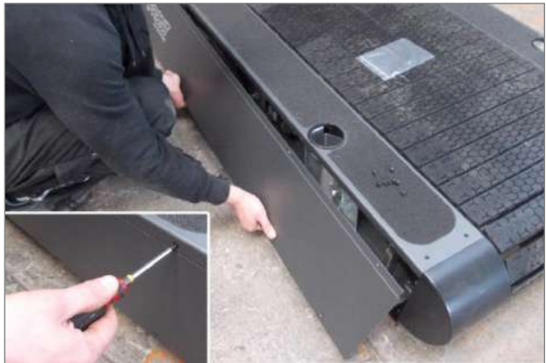
Fig. 15 4Front assembly, side panel
