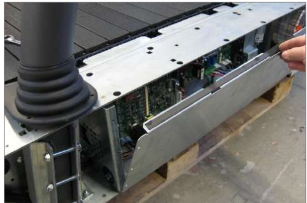
Fig. 29 Desmo assembly, electronic cover plate
