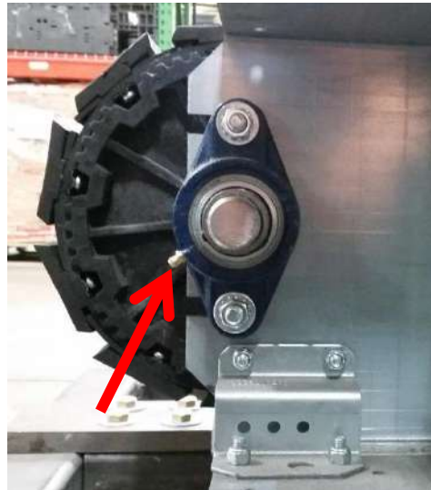
Fig. 114 Lubrication, axle bearing
