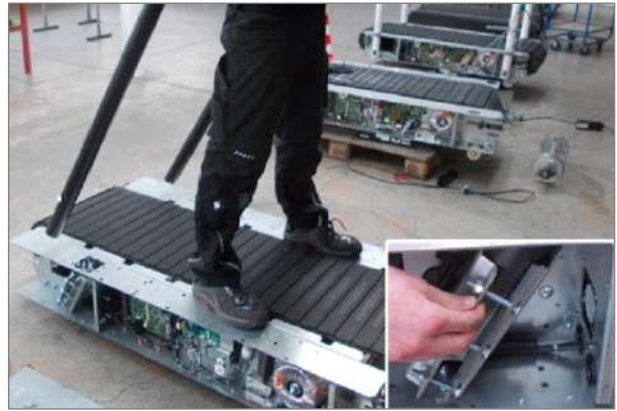
Fig. 40 Mercury/Path assembly, insert tubes
