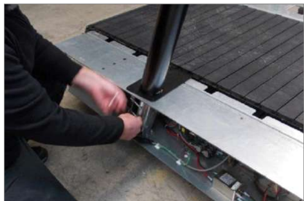
Fig. 53 Pro/Pro XL assembly, insert railing
