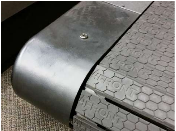
Fig. 50 Mercury/Path assembly, cover plates
