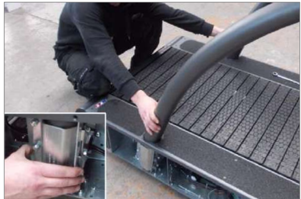
Fig. 18 4Front assembly, inserting tubes
