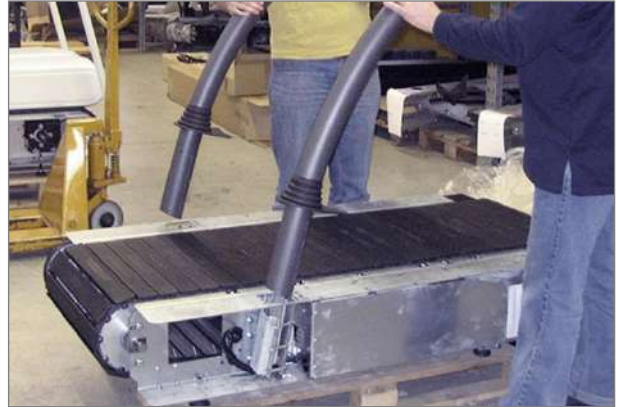
Fig. 27 Desmo assembly, inserting tubes
