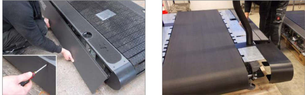
Fig. 14 Removing Side Covers
