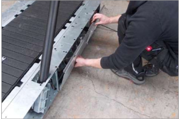
Fig. 42 Mercury/Path assembly, electronic cover plate
