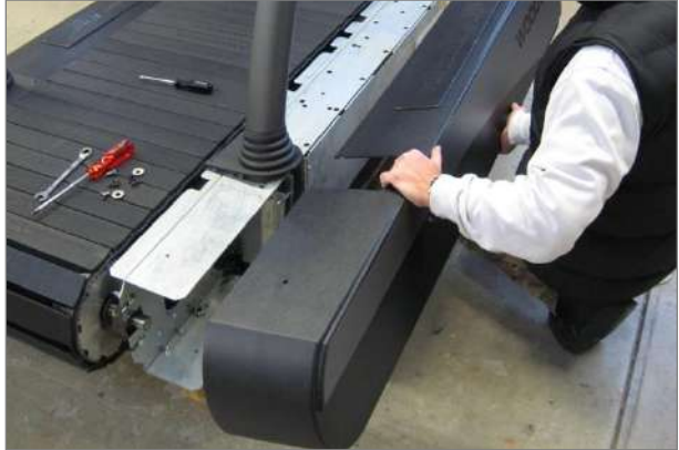
Fig. 24 Desmo assembly, removing side covers
