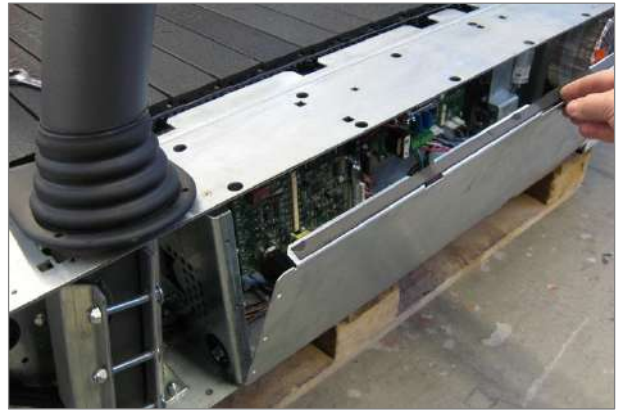
Fig. 34 Desmo assembly, electronic cover plate
