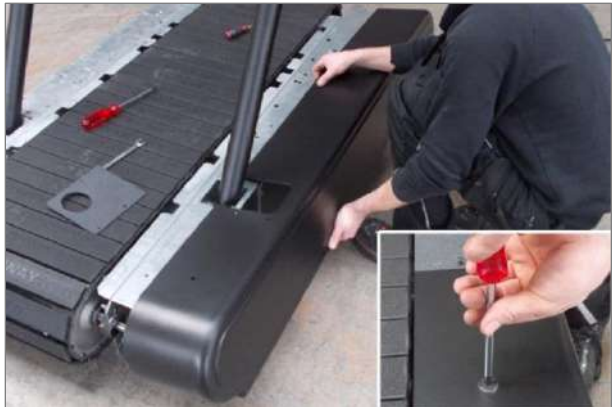
Fig. 37 Mercury/Path assembly, side covers
