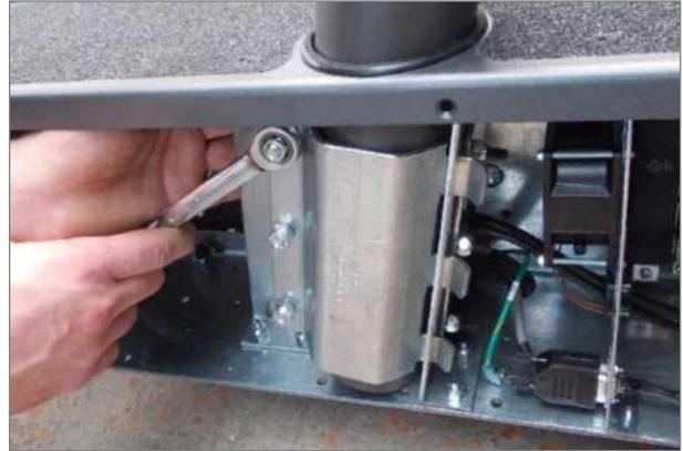
Fig. 22 4Front assembly, securing the railing
