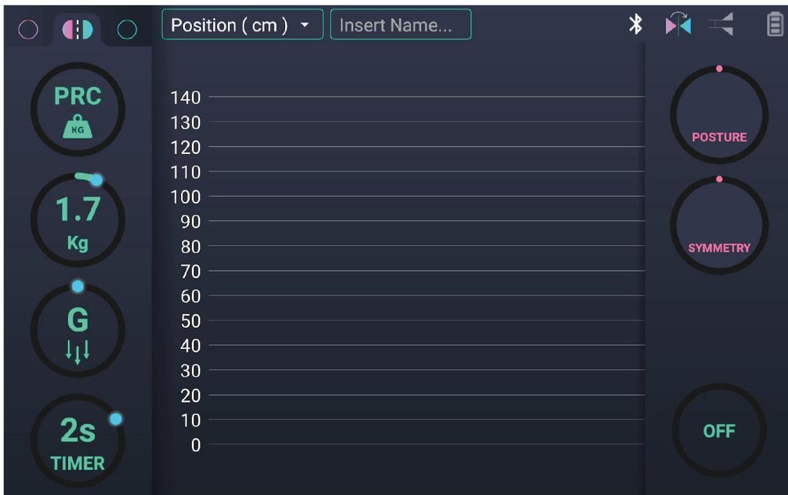
Drag the **Load level** dot around the circle to select loads from 1.0 to 9.9 Kg.
