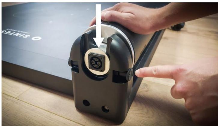
Important: make sure that the two fasteners have clicked in all the way and secure the pin.
