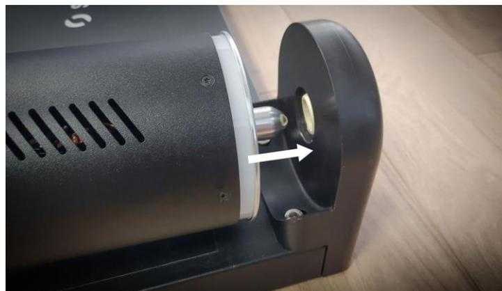
2. insert the quick-release pin on the opposite end of the module into the cavity of the bracket; check that the direction is correct (it can only be inserted in one way). The groove and the two round holes on the pin must face down.
