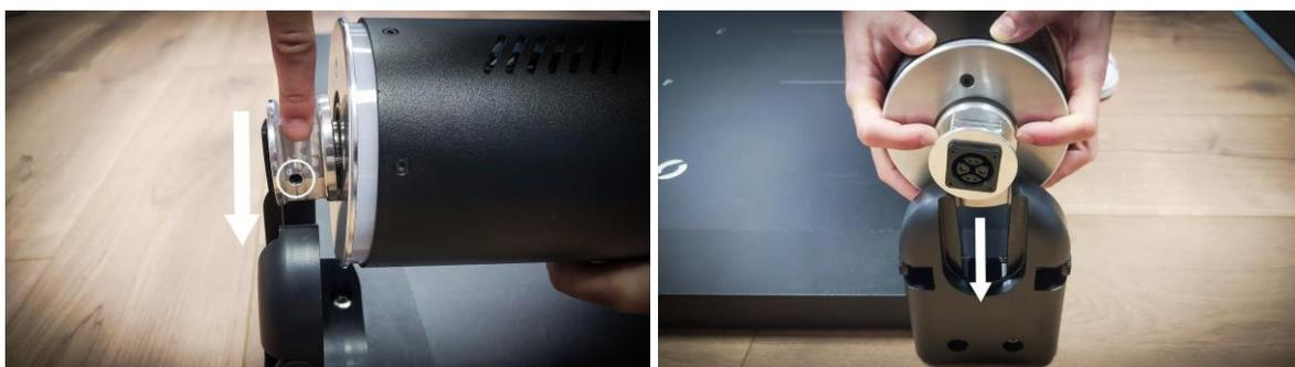
3. Gently push the tubular module down until the two small spring fasteners on the sides of the bracket click in.
