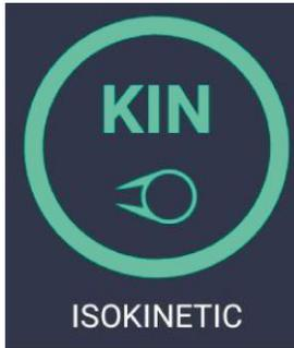
**KIN:** isokinetic load. In this mode you do not set a load (except for maximum load) but the movement speed imposed by the machine. The user will oppose resistance based on his/her strength.
