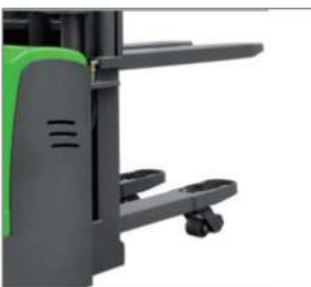
Initial lifting with double-pallet function
