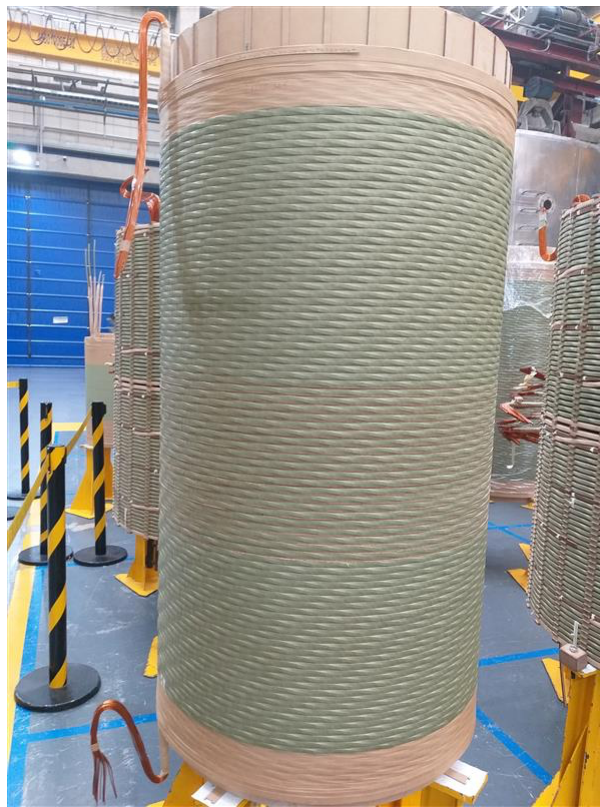
Photo 6: Individual HV winding coil — continuously transposed conductor (CTC) with paper insulation wrapping
