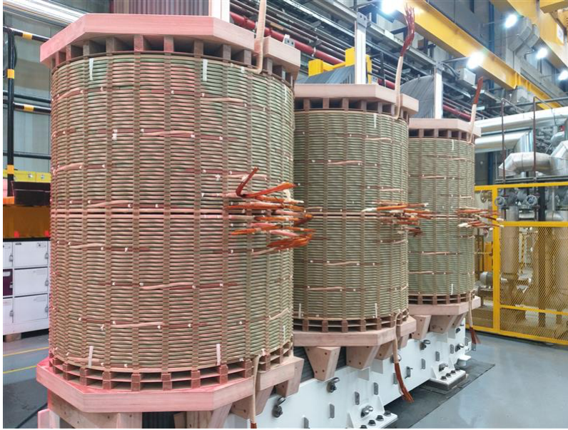
Photo 5: Three-phase winding assemblies — copper disc/helical windings with paper insulation on the manufacturing floor
