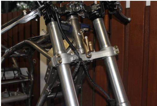
Photo#9 - Front End in place for the time. Steering Damper in place - Mount to be welded in place.
