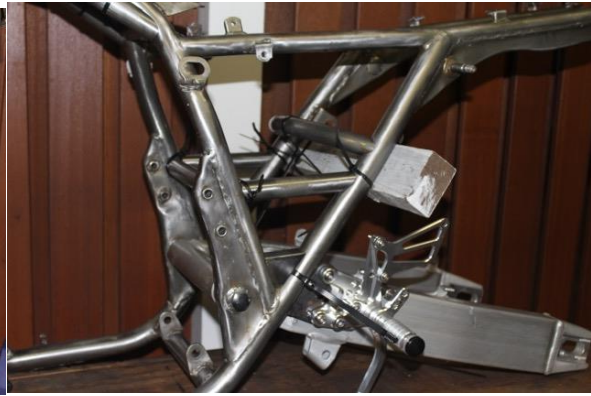
Photo #8 - Rear Set Mounts to be welded.
