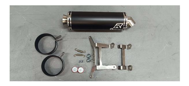
1: install the front support, please use blue Loctite for the M6 screws. Fix it with 12Nm
