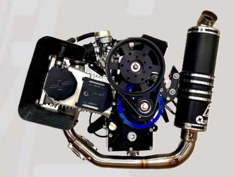
This new cooling shroud is more efficient on a paramotor frame than the current oil cooler system. We have been testing this new system for six months. The tests showed that the cylinder head temperature drops by about 30°C and the oil temperature by about 15°C and it saves 0,7 kg of weight.
