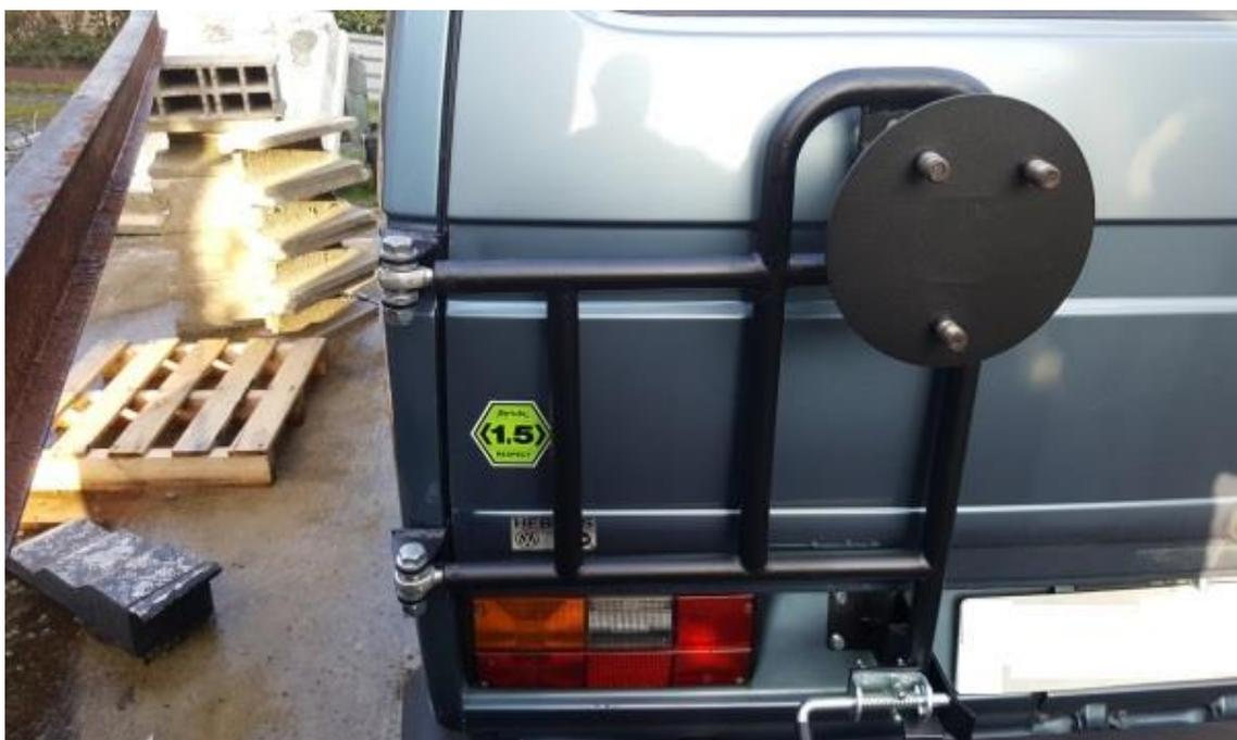
**Now mount the wheel and test. If we see that it drops a little with the weight of the wheel, adjust by turning the**
