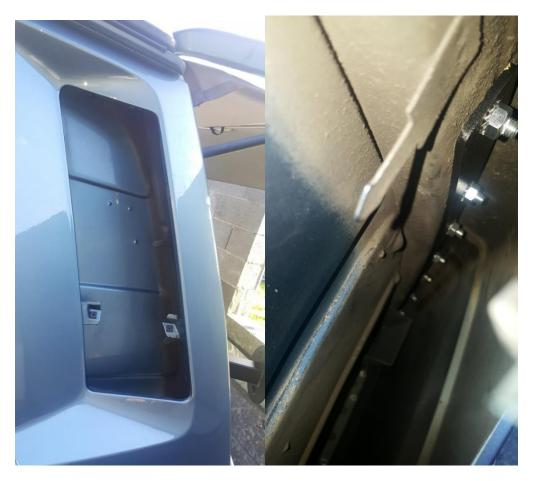
Introduce the fixing plate through the gap of the air inlet
