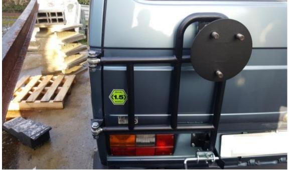
Now mount the wheel and test. If we see that it drops a little with the weight of the wheel, adjust by turning the
