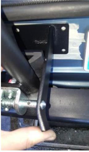
Once straight, present the closure bracket and mark the holes. As before, first protect with tape
