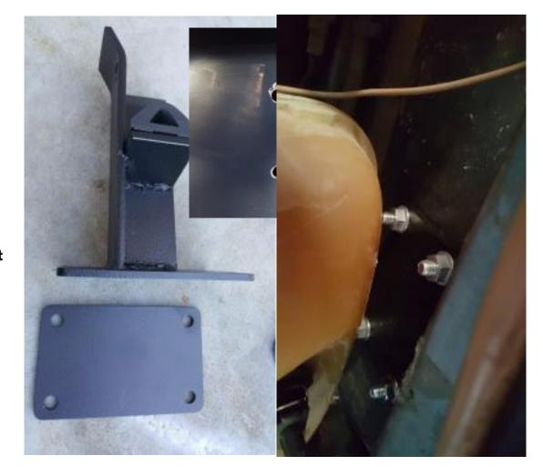
Mount the closure bracket and the internal reinforcement plate
