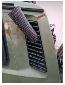
Place the tube on the adapter, the adapter in place, and then the snorkel head.
