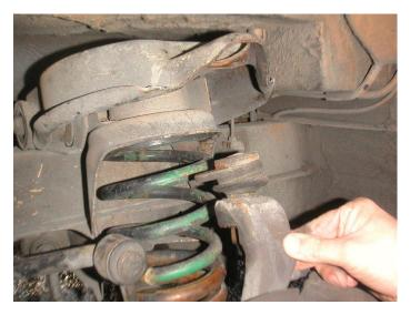
Now we use a little leverage with a bar and remove the spring. We place the supplement on top of the rubber (in the white photo) and insert it again.
