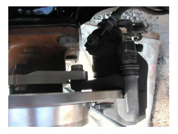
Now you need to put the brake hose in place. There is no problem since they have the same thread. Simply bend the rigid a little, being careful not to make very pronounced curves...
