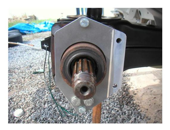
Now we place the ground hub (the diameter must be reduced to 145.9 mm to fit the disc), the disc (we hold it with two nuts) and the caliper.
