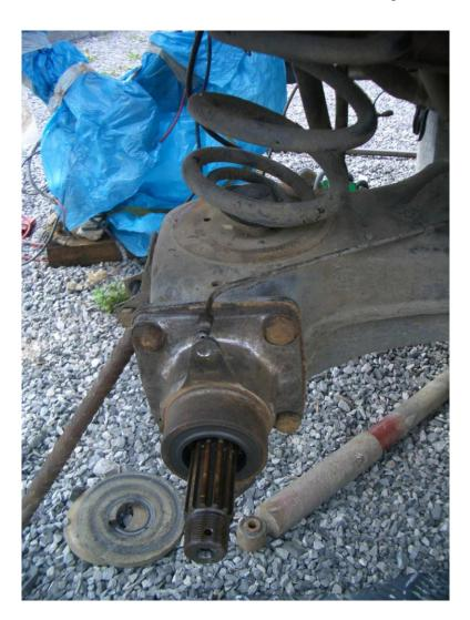
We place the plate (as in the photo) and put the screws: Two M8 with nut and two M10.
