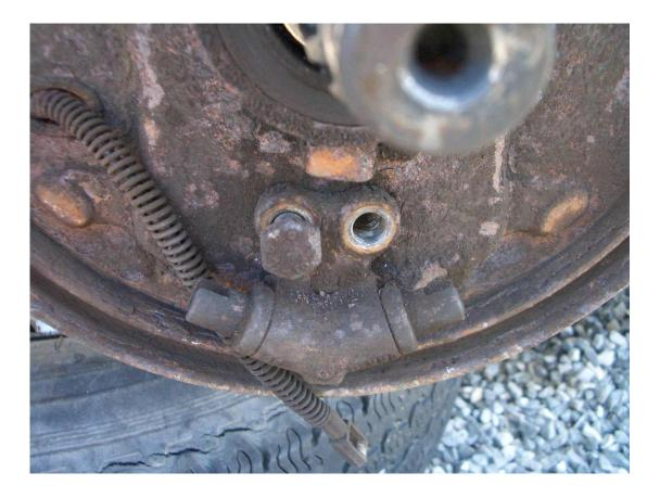
Once this is done, we proceed to tighten the brake hose to prevent leaks. I did it with a few blocks of wood and pliers so as not to damage it.
