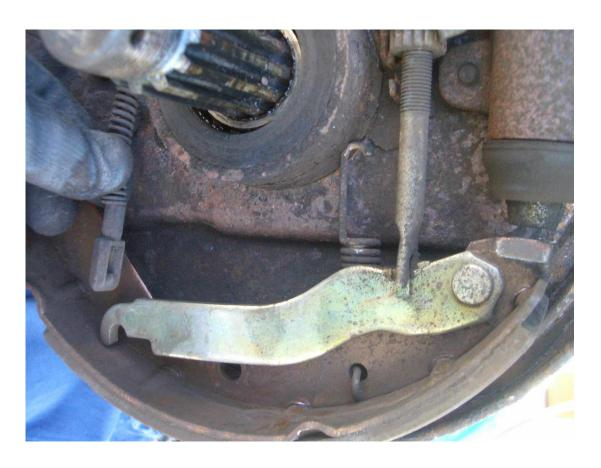
We loosen the handbrake cable, all the springs, the shoes... and leave it as follows:
