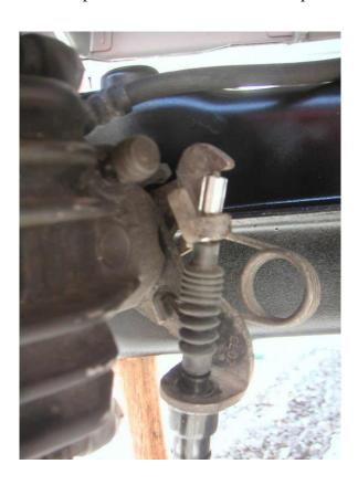
We pass the cable under the suspension arm, fix it with the clip, pass it through its plastic stop guide and bring it to the distributor-tensioner, where we have previously placed a socket, because the new cables are a little longer.
