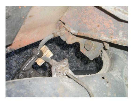
We loosen two screws below, 17 mm wrench
