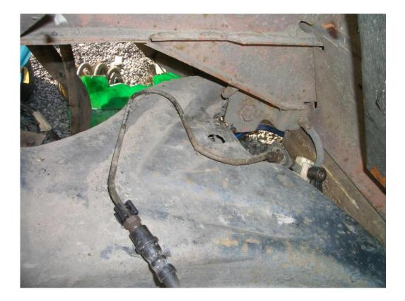
As you can see, the result is very good. Once this is done we can release the pipe. At the end we will bleed the brakes.
