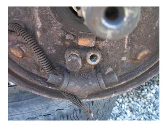
Behind, at the top, we find the rigid. It must be loosened with an 11 mm wrench. Just below there is a 13 mm screw which must be removed to remove the brake cylinder.
