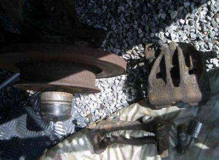
I loosened the caliper by first tightening the hose (see Rear disc assembly), so that the braking circuit does not empty. Once finished, we will purge it to remove air.
