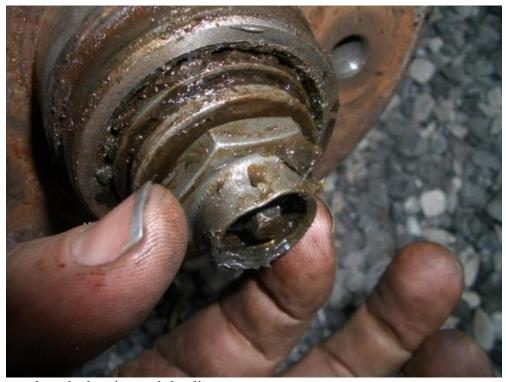
We take out the washer, the bearing and the disc.
