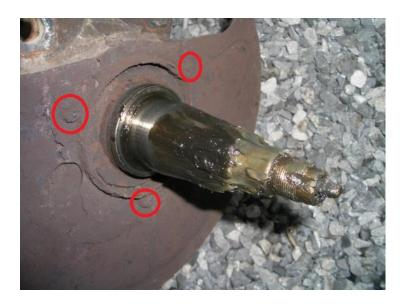
Although it may not seem like it, behind all that rust are three screws holding the drive protector on. We first remove the remaining grease with rags and before starting to work in the area we protect the shaft with a clean cloth to avoid the deposit of impurities which would later affect the bearings. When we are finished working in the area, we will clean everything well and apply lithium grease, especially to the bearings.
