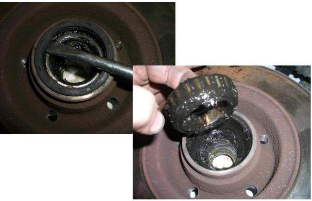
So if we don't change the bearings, we just need to clean them well and change the grease and seal. If we need to change them, we don't do any of that and put the new ones on the turned bushings in the kit.
