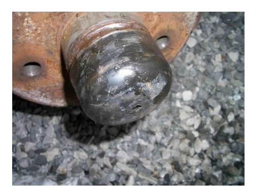
Once this is done, we remove the central nut with a 24 wrench. When we reassemble it, we must tighten the nut just enough to be able to move the washer with a screwdriver (for example). In my case the washer had a lot of play, so it's time to check the bearings...
