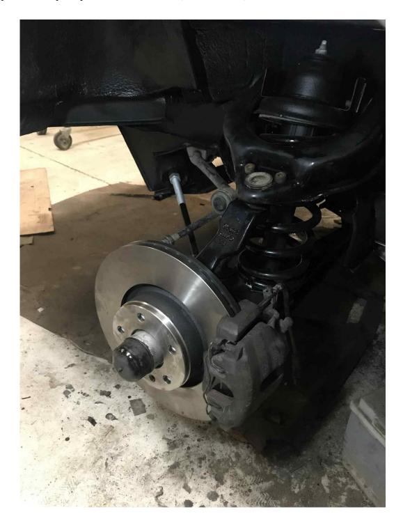
All that remains is to connect the hose (you must use the entire original one, even the rigid section), and adjust the bearings by tightening the nut as I mentioned at the beginning. Once adjusted, a few notches are made in the recesses of the shaft so that it does not come loose.
