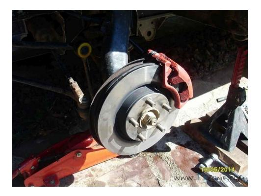
The assembly is very simple. It's like changing discs and calipers normally. You will just have to remember to put the calibrated washers (green arrows) and the new screws.
