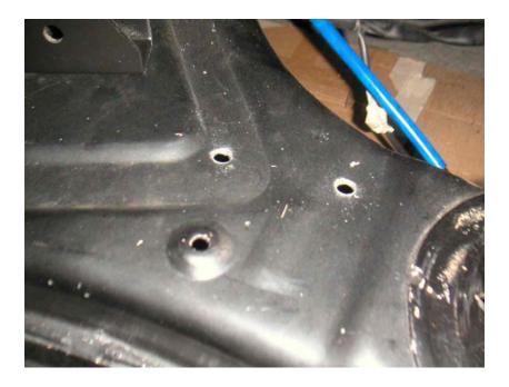
Then we put the fixing plates. We place them in their housing, we put the upper screw, which has a bushing. You have to insert it into a hole in the chassis and then turn it 90° to act as a nut. We block it with a screwdriver or anything else to prevent it from rotating and to be able to tighten.
