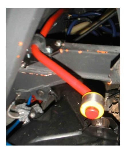
And ready. This is the final assembly. You can see the bolted shock absorber and the 5mm supplement under the lower fixation.
