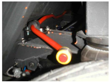
Now we screw the lower fixing, placing the 5mm supplement on the front screw to compensate for the existing depression.
