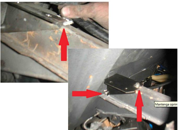
We place the screw that crosses the chassis from one side to the other and tighten it as well. We repeat the process on the other side and half of the work is done.
