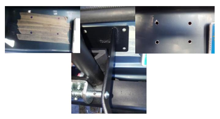
Mount the closure bracket and the internal reinforcement plate
