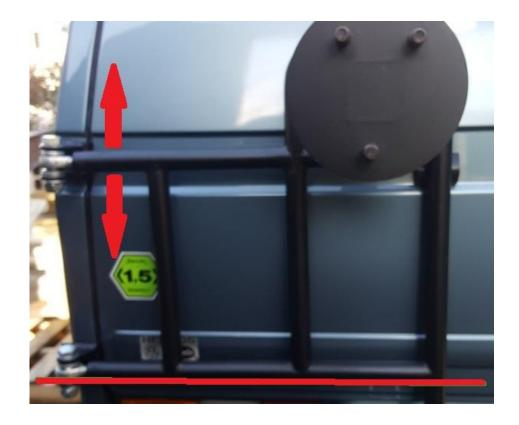
Once straight, present the closure bracket and mark the holes. As before, first protect with tape
