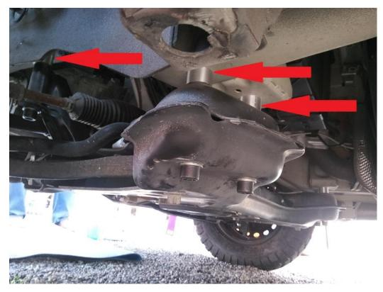
First one side, then the other. The long sockets and screws should be placed on the power steering rack.
