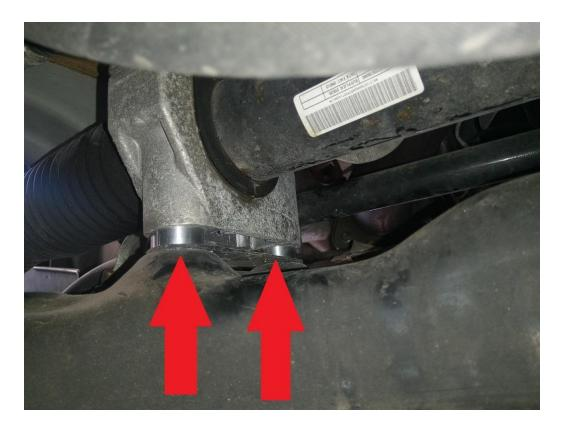
You must loosen the screws, place the rings and screw them back in with the screws included in the kit.
