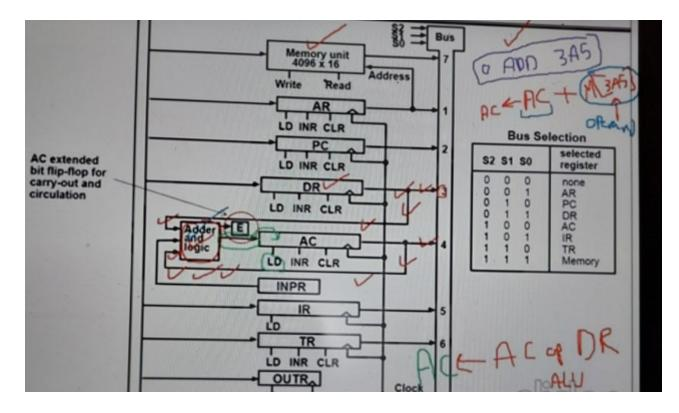
The above drawing depicts a memory unit with 4096 word, each word has 16 bits, below it in order is the Address Register, Program Counter, Data Register, Accumulator, Input Register, Instruction Register, Temporary Register and Finally the Output Register.
