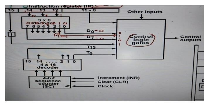
when we wanted to do an operation, it was performed when we had a signal, this circuit is responsible for signals, they enter the clock, and generate signals
