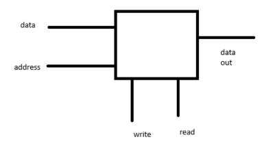
The Memory has a location size that's equal to  $n_1$ , starting from 0 to  $n_1$ -1, each location storing  $n_2$  bits
