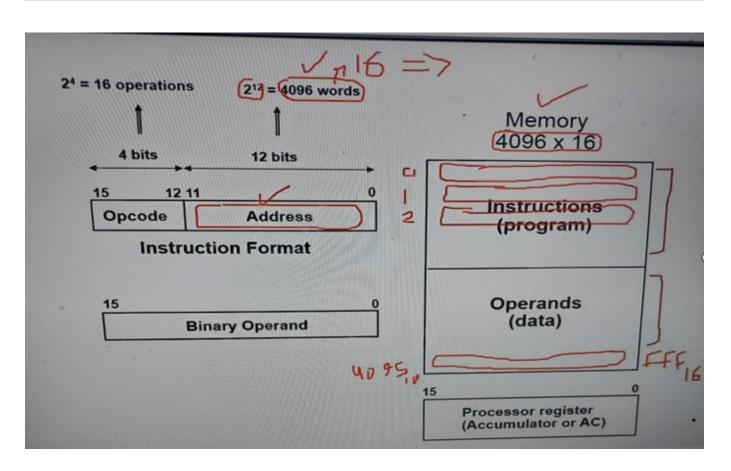
we have a register with 16 bits (from 0-15), from 0-11 is for the address, and the rest for the opcode, subtract 1 bit from the opcode for other stuff, leaving it with 3 bits, where we can do 8 operations with it, we also have 4096 locations in the memory (as we have 12 bits for the address).
