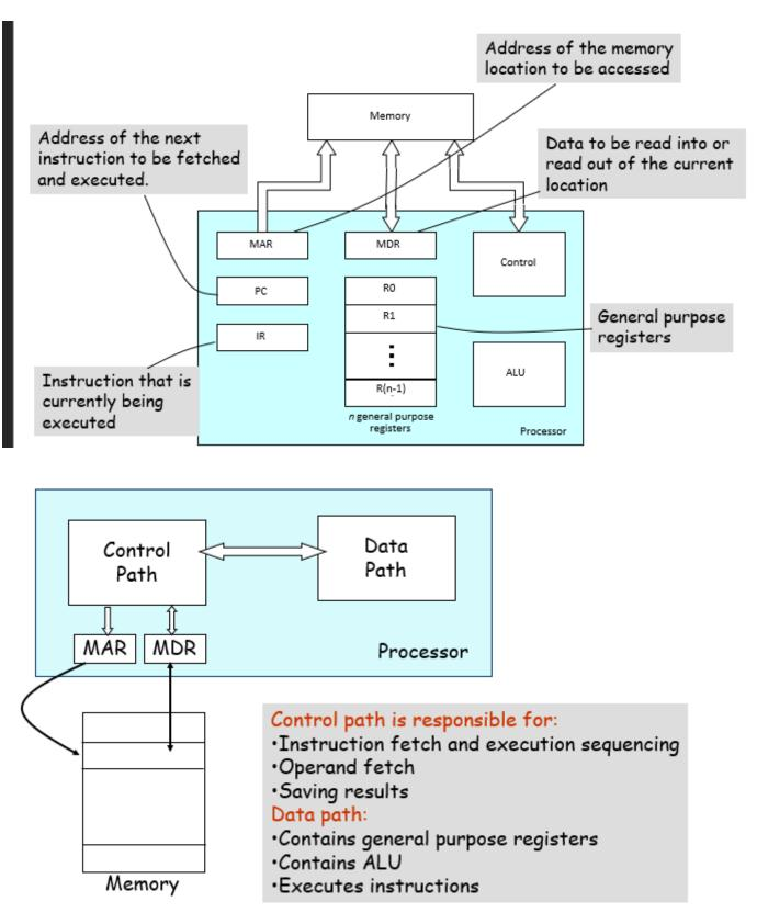
Basic processor architecture has several registers to assist in the execution of the instructions.
