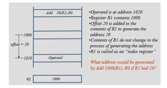
The effective address is calculated by adding a constant offset to the contents of a specified register.
