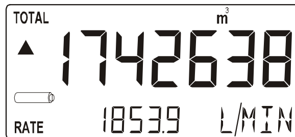
Fig. 5: Example of low-battery alarm
