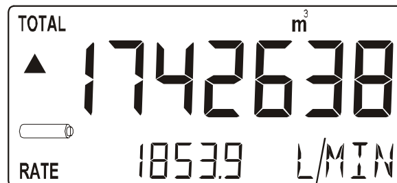
Fig. 5: Example of low-battery alarm
