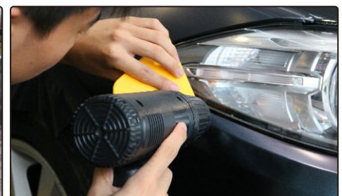
3. Use squeegee and heat gun to make it flat
