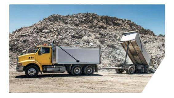
**TAILGATES**: HH vehicles have air operated tailgates with warning labels attached. Drivers need to keep well away from tailgates during operation of air rams.
