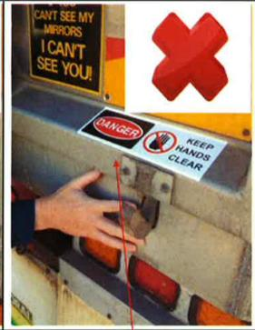
Before exiting the cab ensure the tailgate lever is in the open position and no one else will be inside the cab moving the tailgate lever to the closed position without the drivers knowledge
