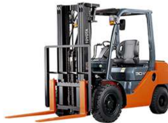
Diesel Forklift 3-10 ton 2 & 3 stage mast with 3 to 6m Lift height Options
