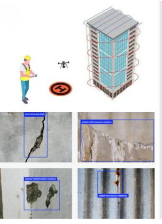
Drones have the ability to capture high-resolution images and data from hard-to-reach areas, drones are proving to be a valuable tool for infrastructure inspections. From bridges and buildings, drones are helping to identify potential issues before they become major problems. Building inspection with drones is becoming an increasingly popular method for conducting infrastructure inspections, as it allows for more efficient and comprehensive assessments of buildings and other structures.
