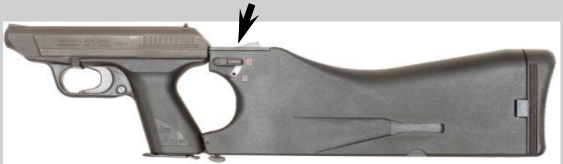
Figure 20: HK VP-70Z pistol with stock holster. The arrow indicates the fire mode selector.
