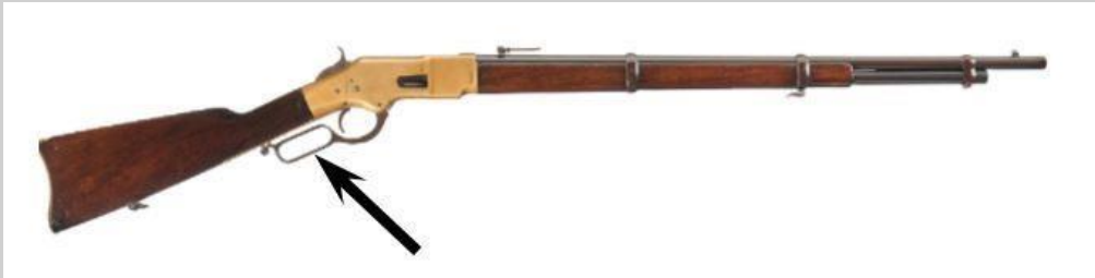
Figure 5: Winchester carbine model 1866. The arrow indicates the manual repeat trigger lever.
