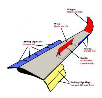
Several key parts make an <u>airplane wing</u>. These parts work together to ensure flight stability is maintained, lift is generated, and the flight is controlled.
