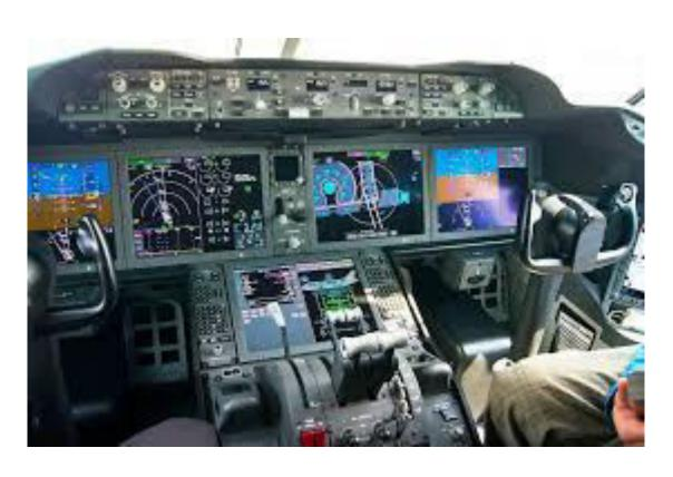
The cockpit includes a seating area for the flight crew, flight instruments, avionics, audio/radio communications, and flight controls.
