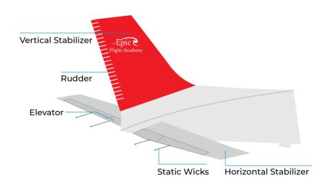
The empennage, also called the tail or tail assembly, is located at the rear of an airplane.
