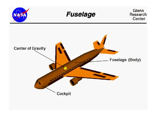
The **fuselage**, or body of the airplane, is a long hollow tube which holds all the pieces of an airplane together.
