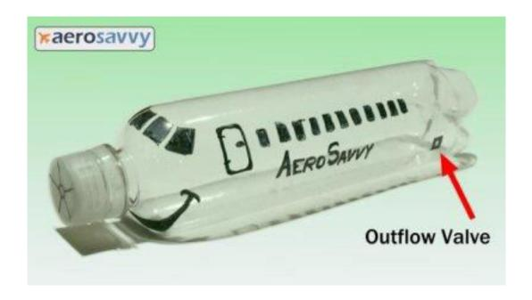
A fuselage is a bit like a cigar tube with a hole in the back: the pressurization systems constantly pump compressed air from the compressors that are present in the engines.
